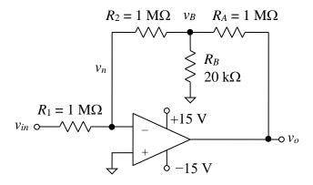
2. Show that the op-amp in the circuit diagram below saturates at one of the power supply voltages, and find the resulting voltages v and  $v_o$ . Note that the circuit is not a diff amp because  $R_4/R_3 \neq R_2/R_1$ , not even approximately. You may ignore the minor effects of the input offset voltage and input bias currents of the op-amp. Assume that  $v_o$  can swing all the way from -10 V to +10 V.
