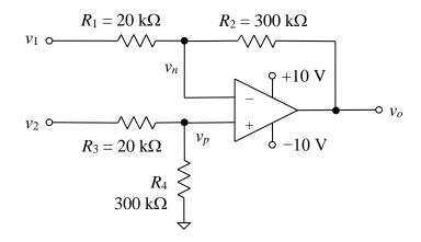
5. Find the output voltage for the diff amp in the previous problem if the single-ended input voltages are  $v_1 = 680 \text{ mV}$  and  $v_2 = -240 \text{ mV}$ . Find the node voltages  $v_n$  and  $v_p$  as well. Be careful! Continue to assume that the op-amp is ideal and that the resistors have the exact values shown.
