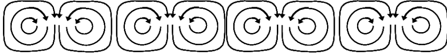
FIG. 1: Schematic of a chain of alternating vortices. The arrows show the direction of the flow within each vortex.
