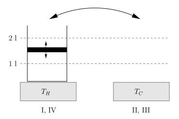
Consider the following cyclic thermodynamic process with a container containing 1 mole of an ideal gas. (This discussion is meant to be a complement to the discussion of the Carnot cycle in Section 19.2 of your text. The p-V diagram for this process is on the following page. The cycle starts with the gas contained in a 11 volume at equilibrium with a temperature bath at  $T_H = 600$  K; this is point **A** in the p-V diagram. The gas then undergoes four thermodynamic processes:
