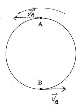
$$\vec{q} = \frac{\Delta \vec{V}}{\Delta t} = \frac{\vec{V}_B - \vec{V}_A}{\Delta t} = \frac{(6m/s 2) - (-6m/s 2)}{0.55}$$
