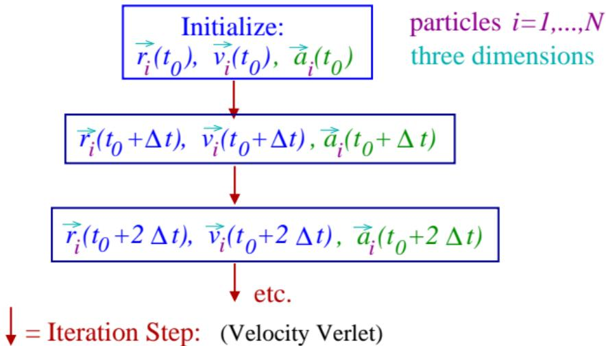
$$\boxed{\begin{aligned}\vec{r}_i(t+\Delta t) &= \vec{r}_i(t) + \vec{v}_i(t)\Delta t + \vec{a}_i(t)(\Delta t)^2/2 \\ \vec{v}_i(t+\Delta t) &= \vec{v}_i(t) + (\vec{a}_i(t) + \vec{a}_i(t+\Delta t))\Delta t/2 \\ \vec{a}_i(t) &= \vec{F}_i(t)/m_i = -\vec{\nabla}_{\vec{r}_i} U(t)/m_i\end{aligned}}$$
