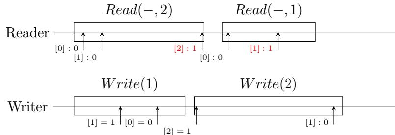
We can resolve this issue with a *one-sided clear*: observe that we do not need to clear higher indices, as  $Read$  stops when it first sees a 1.  $Reads$  could still be returning stale values, though, as a  $Write$  could have set a lower bit, which the  $Read$  already passed. Thus,  $Read$  can search until it finds a 1, then search back down to see if a smaller value has been written since, and return the smallest value it sees.
