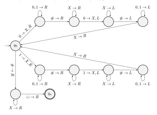
Note that we do not draw all, or in this case any, transitions to  $q_{reject}$ . Since TMs are deterministic, there must be an edge from every state on every possible tape symbol, which can be a **lot** of edges. For clarity, any edges not drawn are considered to go to  $q_{reject}$ , where the TM immediately halts and rejects the input.
