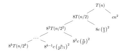
We can now solve for the number of levels, k. The base case is assumed to be T(1) = O(1), so we need to find k s.t.  $n/2^k = 1$ . This is true when  $k = \log_2 n$ . Substituting this into the exponent of the coefficient 8, we get  $8^{\log_2 n}O(1) = O(n^3)$  for the recursive portion of the runtime.
