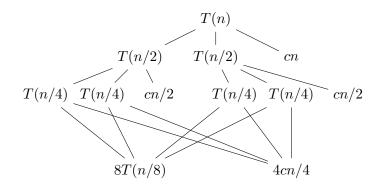
Note that each node in the tree is either replaced by substituting the recurrence again or is non-recursive (closed form). If we add all the leaves, we will get the total value of the function.
