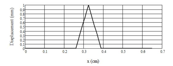
The locations that correspond to the start, peak, and stop points of the triangular section are x = 0.4L, x = 0.5L, and x = 0.6L, respectively, where L is the length of the string.
