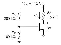
By the way, temperature sensitivity is one reason why the circuit considered in this problem is never used in practice to bias a MOSFET. A resistor (usually labeled  $R_S$  in Sedra & Smith) added in series with the source terminal greatly stabilizes the drain current against temperature changes.
