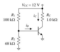
2. For the circuit shown below, find the quiescent collector voltage  $V_C$ , the quiescent emitter voltage  $V_E$ , and the quiescent collector current  $I_C$ . Assume that  $\beta = 150$ ,  $V_{CE}|_{\text{sat}} = 0.2 \text{ V}$ , and that the base-emitter (BE) junction can be modeled using a constant voltage drop of  $V_F = 0.7 \text{ V}$ . Also find the region of operation of the BJT.
