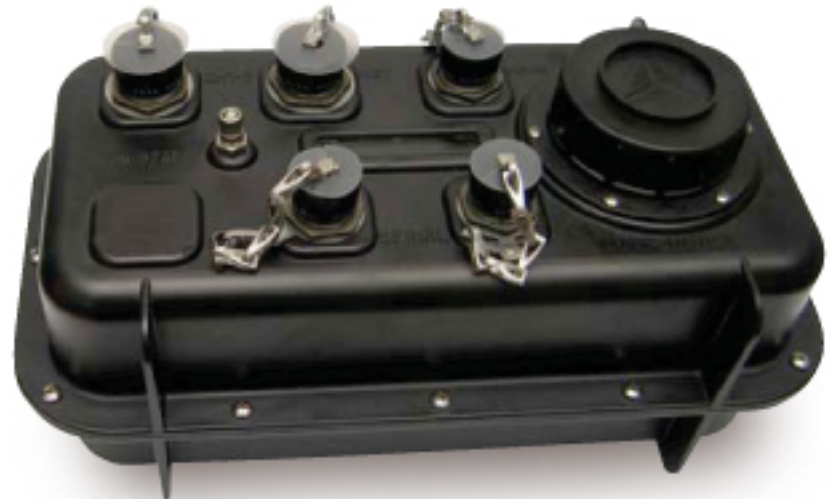
Reftek 130: An existing seismic collection device
