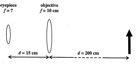
a) Determine the focal length of the eyepiece. Show all work.
