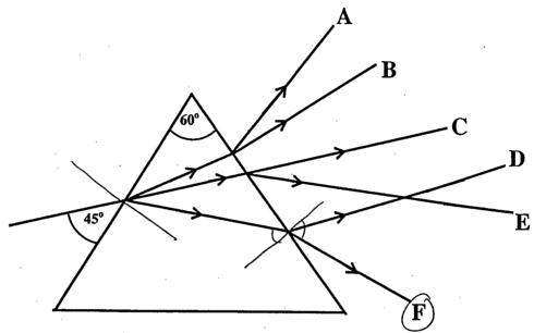
when passing from a material of lower n to higher n the ray is bent towards the normal => E or F.
